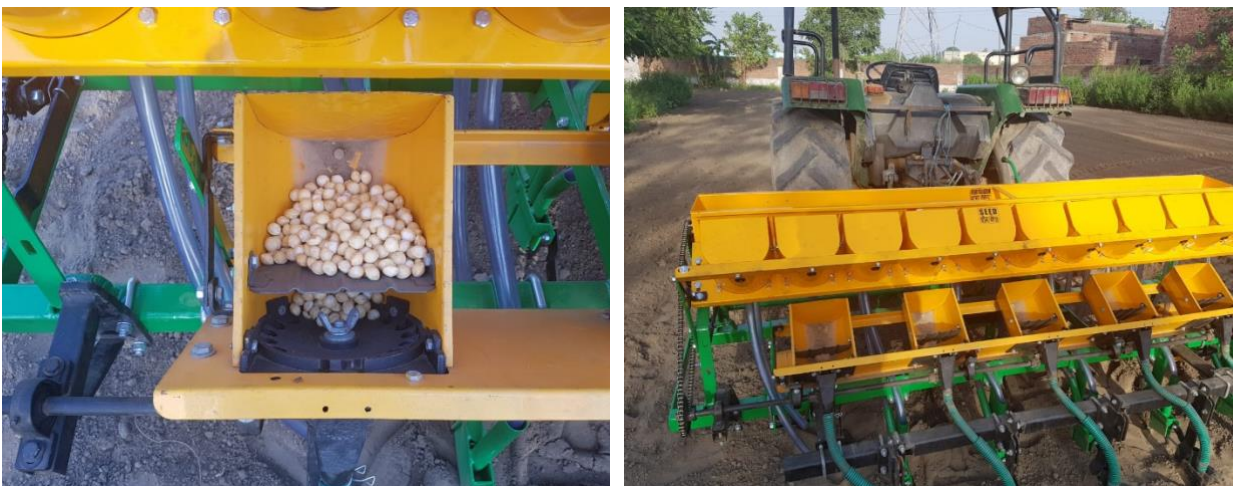
Figure 17. Mechanized applicator for subsurface fertilizer application and seeder
