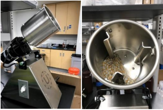
Figure 21. Tabletop seed coater (a); and loaded drum (b).
