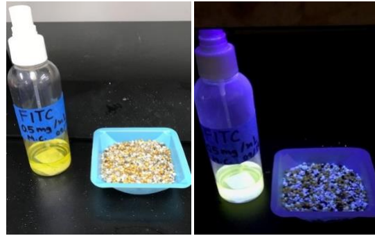
Figure 22. FITC solution and fertilizer mix under natural light (left); and UV-light (right).
