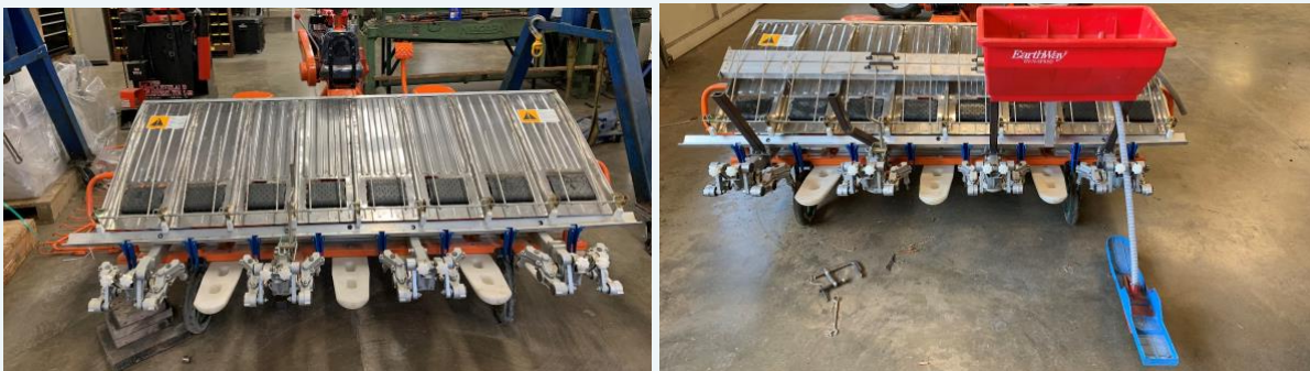
Transplanting unit (left) and the UDP application device with the hopper attached to the transplanter (right).
