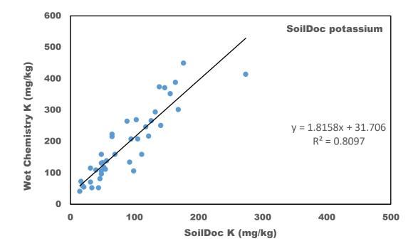
Figure 19. Results of the Exchangeable Potassium Analysis of 40 Archived Soil Samples Determined with the SoilDoc Soil Test Kit as Compared with Values Obtained from Wet Chemistry
