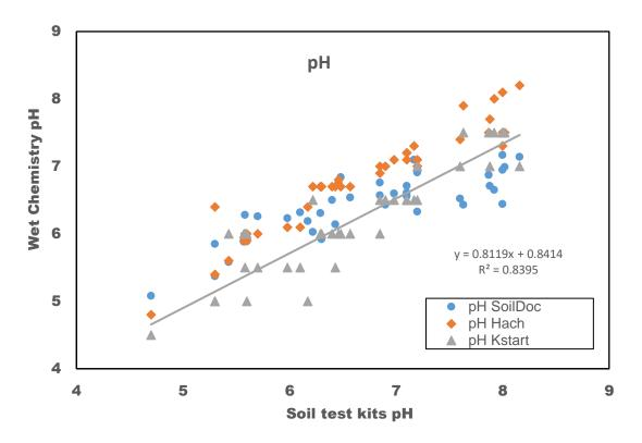
Figure 12. Results from the pH Analyses of 40 Archived Soil Samples Determined with the Portable Soil Test Kits as Compared with Values Obtained from Wet Chemistry
