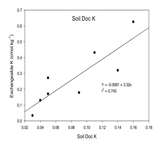
Figure 9.Results from the Exchangeable Potassium Analyses from the SoilDoc Soil<br/>Test Kits as Compared with Values Obtained from Wet Chemistry
