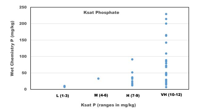
Figure 18. Results of the Available Phosphorus Analysis of 40 Archived Soil Samples Determined with the Kasetsart Soil Test Kit as Compared with Values Obtained from Wet Chemistry
