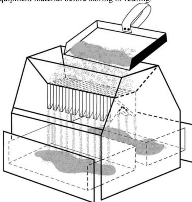
**Figure A.4. A Riffle Splitter with 20 Chutes and Two Collecting Pans**
