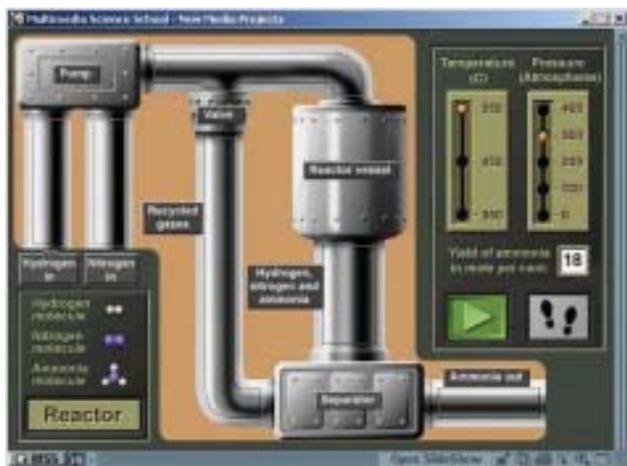
This was a revolutionary moment in human history. The Haber-Bosch system, as it is called now, used far less energy than the competing methods, Birkeland's flaming discs or Washburn's cyanamid process. The Haber-Bosch reaction creates a certain amount of heat on its own, which is used to preheat the gases, lowering energy costs. They worked continuously, day and night, gases in, ammonia flowing out.
