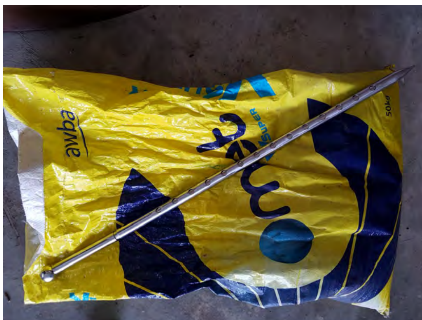
Figure 1. Prototype of sampling probe made of stainless steel.
