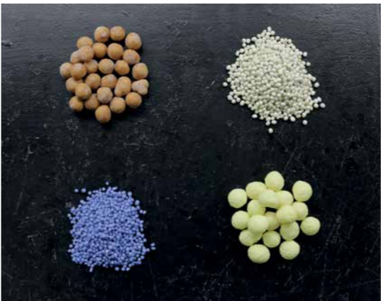
Four kinds of coating: zinc oxide and rice-bran wax (top left), gypsum (top right), polymer (bottom left), sulphur (bottom right)
