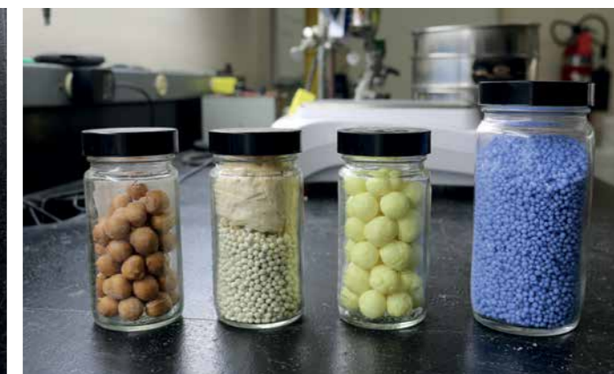
(left to right) Zinc oxide and rice-bran wax, gypsum, sulphur, and a polymer are all types of coatings that control the release of nitrogen or other elements into the soil
