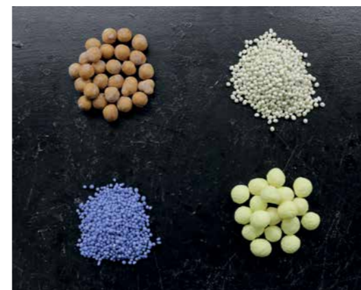
Four kinds of coating: zinc oxide and rice-bran wax (top left), gypsum (top right), polymer (bottom left), sulphur (bottom right)
