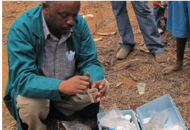
▲ Soil testing using a portable soil test kit in a farmer's field in Rwanda
