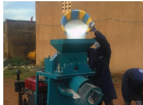
Photo 7. Production of Urea Briquettes
