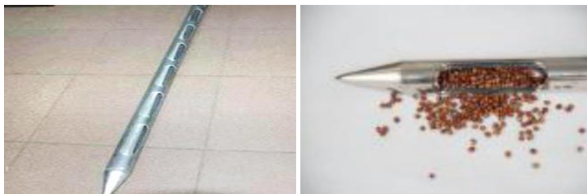
Figure 12. Double Tube Trier in open and closed positions
