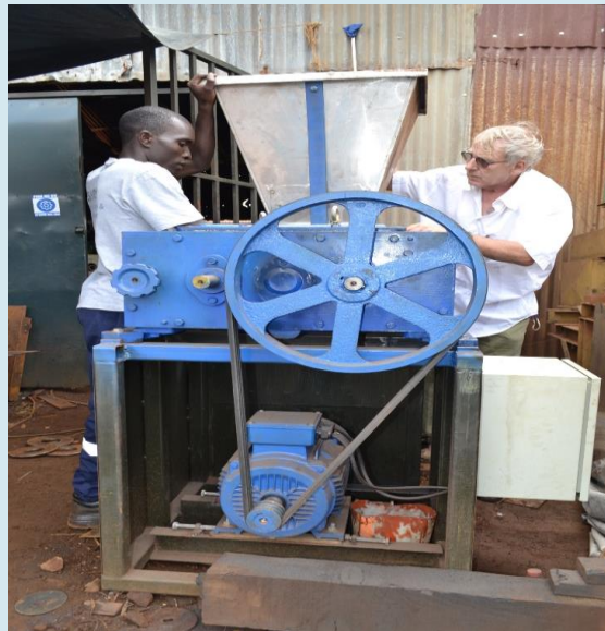
High powered briquetting machine under development in Ndeeba, Kampala, Uganda
