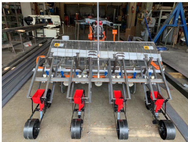
Figure 7. Rice transplanter-deep placement applicator development at Mississippi State University
