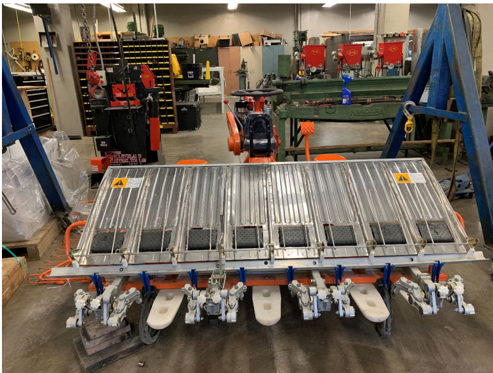
Figure 14. Procured Machine Showing the Transplanting Unit Where the UDP Application Units Will Be Attached
