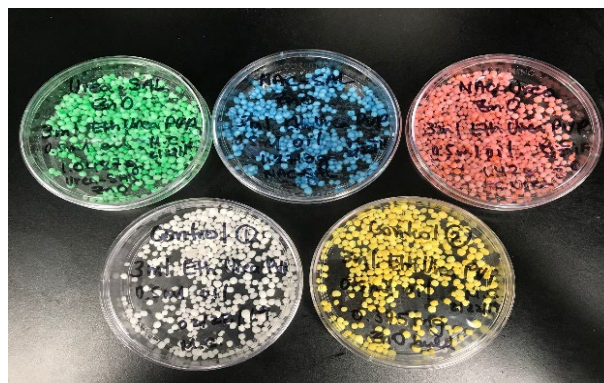
Figure 6. Urea Coated with Urea-SAL ZnO (green), NAC-SAL ZnO (blue), NAC-Urea ZnO (red), Bulk ZnO (yellow), and Control Mix (white)
