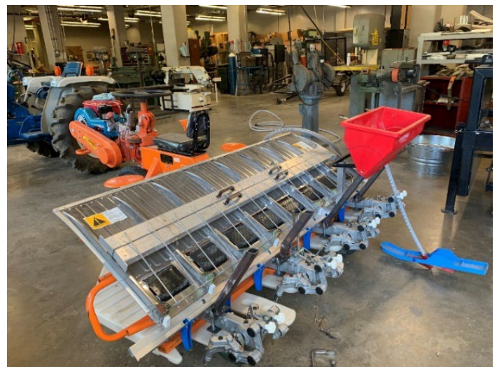
Figure 6. FDP application device, with the hopper attached to the transplanter (side view).
