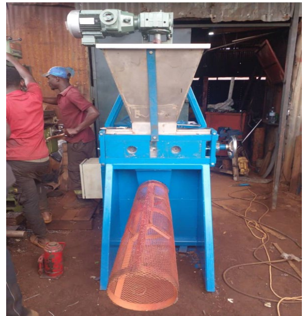
Figure 5. Large-scale briquetter machine built in Kampala.
