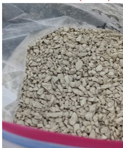
Figure 34. Processing of as-received Tahoua natural phosphate rock (PNT) to compacted 75TNP:25MAP product for field trials.
