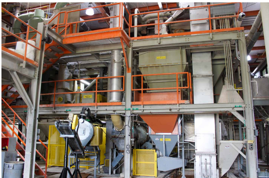
The Large Scale Granulation Pilot Plant at IFDC's Muscle Shoals research center validates innovative production processes
